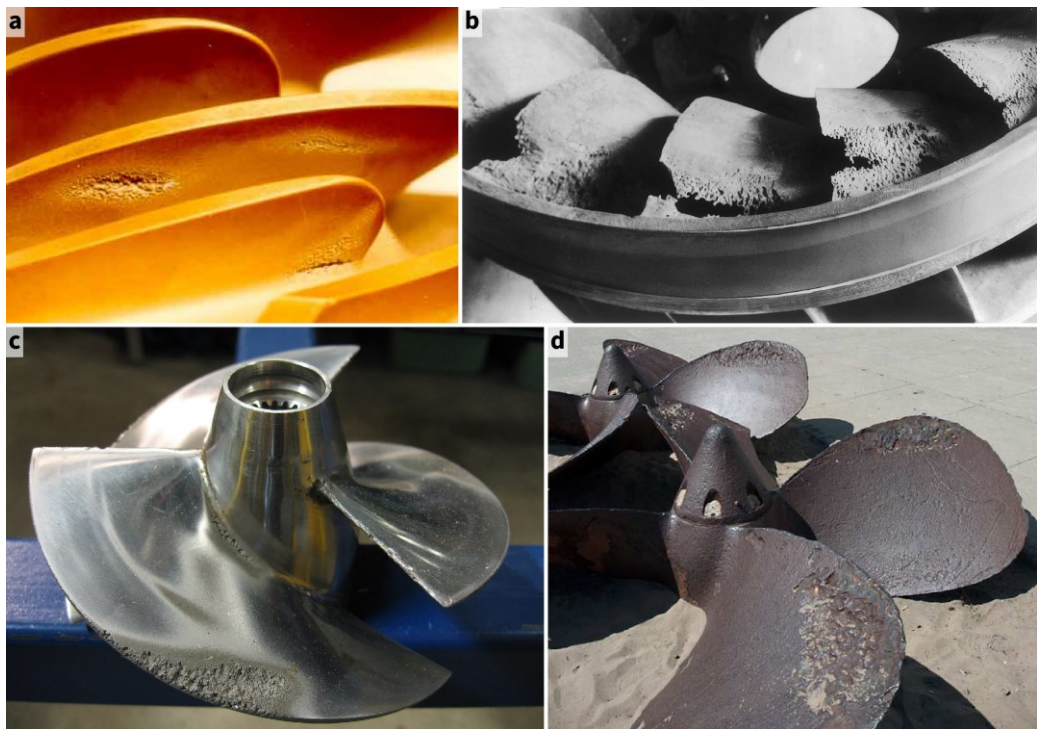
Fig. 2.5 – Cavitation erosion on different components. a, The blades of a mixed flow pump impeller [2]; b, The blades at the discharge of a Francis turbine [49]; c, The blades of the propeller of a personal watercraft [50]; d, The blades of the propeller of a vessel [51].
