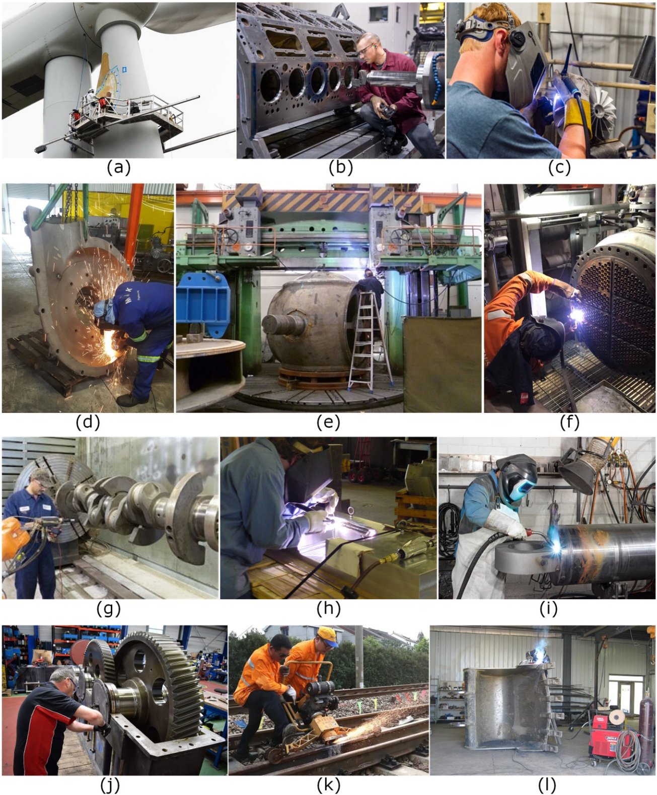
Figure 1.1 Components that are in repair process: (a) turbines, (b) engine blocks, (c) compressors, (d) pumps, (e) valves, (f) heat exchangers, (g) crankshafts, (h) moulds, (i) hydraulic cylinders, (j) gear boxes, (k) rail tracks, and (l) buckets.
