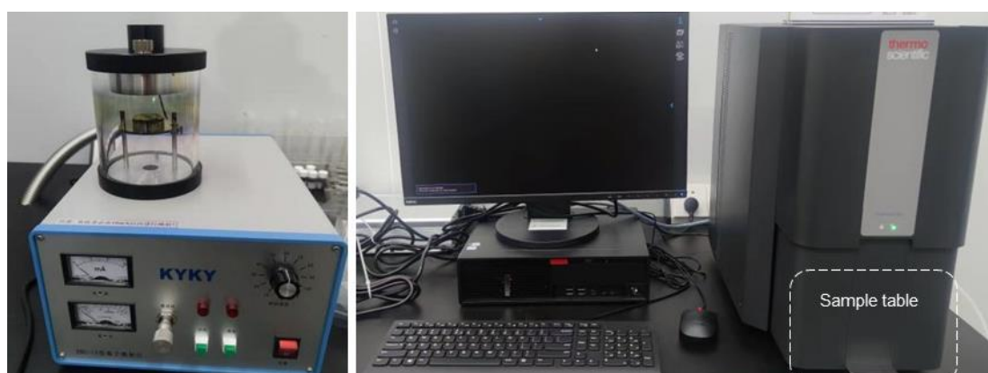
Figure 3. 3 SEM gold spraying equipment (left) and test machines (right).
