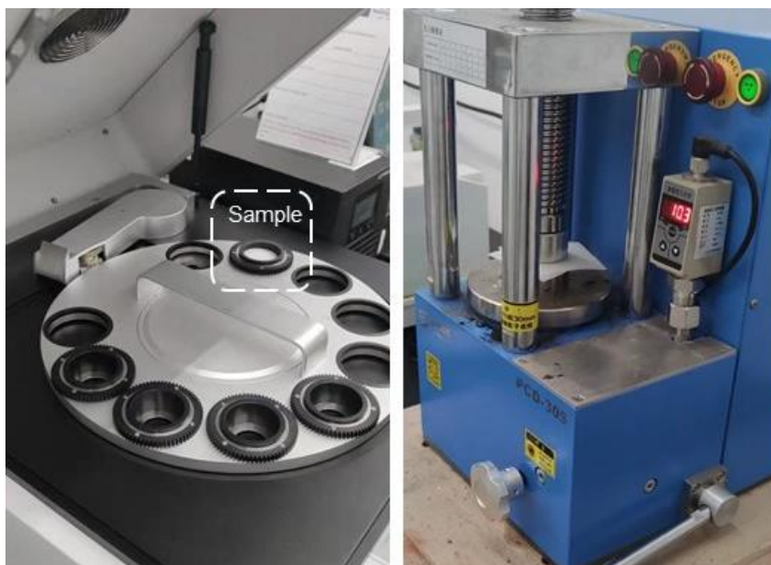
Figure 3. 4 XRF test equipment (left) and tablet press machine (right).
