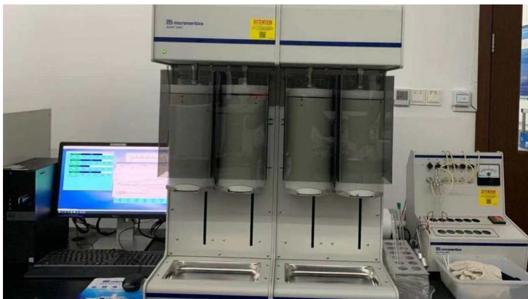
Figure 3. 6 The images of BET, test equipment (left), and degas equipment (right).
