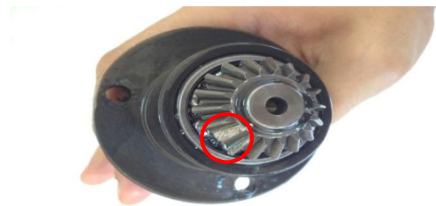
Figure 2. The gear with faulty tooth.
