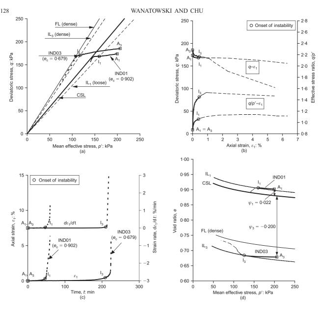
Fig. 8. Effect of void ratio on instability of sand under drained conditions: (a) effective stress paths; (b) deviatoric stress and effective stress ratio against axial strain; (c) axial strain and volumetric strain against time; (d) e-p' plots
