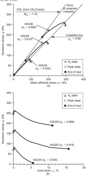
Fig. 4. Definition of instability line and zone of potential instability based on  $CK_0U$  plane-strain tests on very loose sand: (a) effective stress paths; (b) corresponding stress-strain curves
