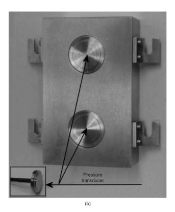
Fig. 2. Plane-strain apparatus: (a) photograph of elevation; (b) photograph of vertical platen (after Wanatowski & Chu, 2007)
