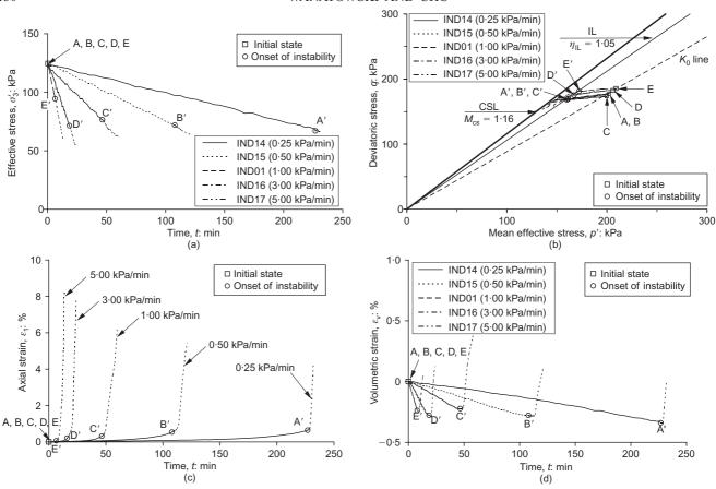
Fig. 10. Effect of  $\sigma'_3$  reduction rate on instability of very loose sand: (a)  $\sigma'_3$  against time; (b) effective stress paths; (c) axial strain against time; (d) volumetric strain against time
