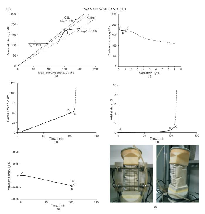
Fig. 14. Instability behaviour of very loose sand under drained/undrained conditions (Test IND24,  $e_c = 0.903$ ): (a) effective stress path; (b) stress-strain curve; (c)  $\Delta u$  against time; (d)  $\varepsilon_1$  against time; (e)  $\varepsilon_v$  against time; (f) specimen at end of test (A, start of instability test; B, onset of instability; C, closure of drainage valves)
