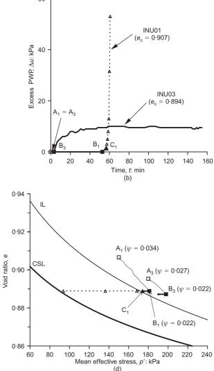
Fig. 5. Instability of loose sand under undrained condition: (a) effective stress paths; (b) excess pore water pressure against time; (c) axial strain against time; (d) e-p' plot
