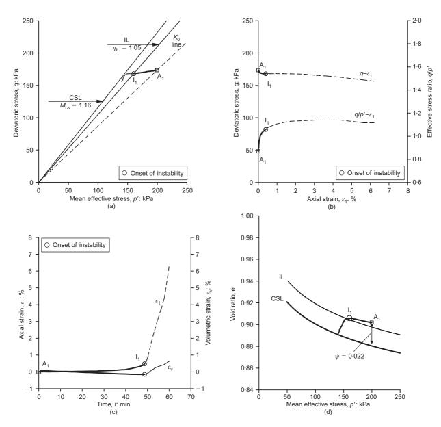
Fig. 6. Instability of loose sand under drained condition (Test IND01,  $e_c = 0.902$ ): (a) effective stress path; (b) deviatoric stress and effective stress ratio against axial strain; (c) axial strain and volumetric strain against time; (d)  $e_{-p'}$  plot
