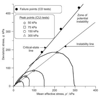
Fig. 3. Definition of instability line and zone of potential instability based on CIU triaxial tests on loose sand
