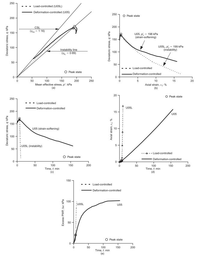
Fig. 15. Comparison of undrained tests conducted on very loose sand under deformation-controlled and load-controlled loading modes: (a) effective stress paths; (b) stress-strain curves; (c) deviatoric stress against time; (d) axial strain against time; (e) excess pore water pressure against time
