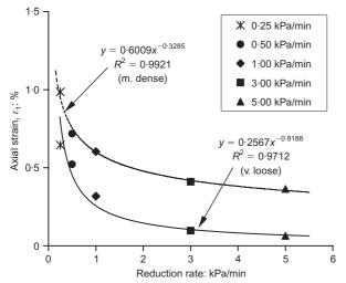
Fig. 12. Relationship between axial strain developed in CSD test and  $\sigma'_3$  reduction rate
