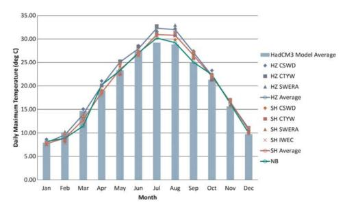
Figure 3. Comparisons of daily maximum temperatures of weather years in Hangzhou, Shanghai and Ningbo with equivalent HadCM3 data.
