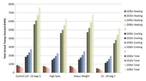
Figure 16. Comparison of heating and cooling demands for the 'control' office room in Ningbo with varying building specification, building 'weight' and a wider internal comfort temperature range.
