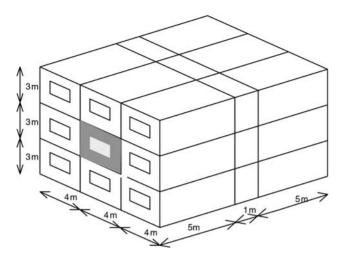
Figure 10. Office room (shaded) to be simulated in the second-order model.
