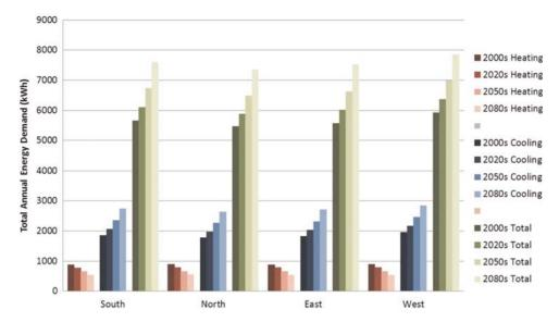
Figure 14. Comparison of heating and cooling demands for the 'control' office room in Ningbo with varying glazing orientations.
