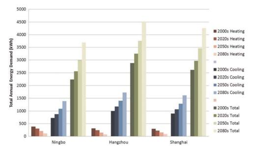
Figure 19. Comparison of heating and cooling demands for optimized configurations with north-facing glazing for Ningbo, Shanghai and Hangzhou.
