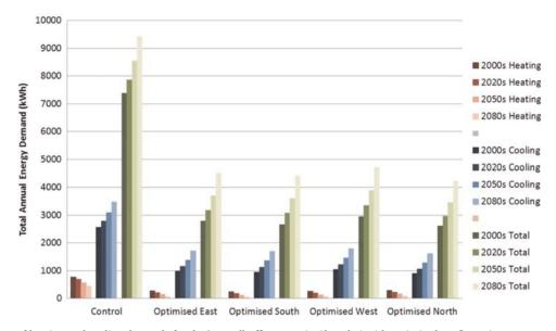
Figure 18. Comparison of heating and cooling demands for the 'control' office room in Shanghai with optimized configurations.
