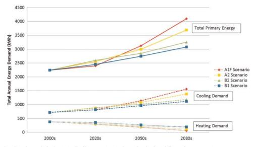
Figure 20. Heating and cooling demands for 'optimized' office room in Ningbo under the four different future scenarios.
