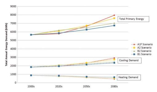
Figure 12. Heating and cooling demands for the 'control' office room in Ningbo.
