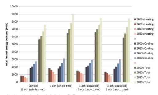
Figure 15. Comparison of heating and cooling demands for the 'control' office room in Ningbo with varying air-change rates.
