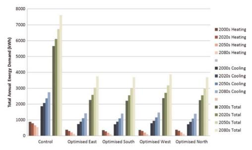
Figure 17. Comparison of heating and cooling demands for the 'control' office room in Ningbo with optimized configurations.
