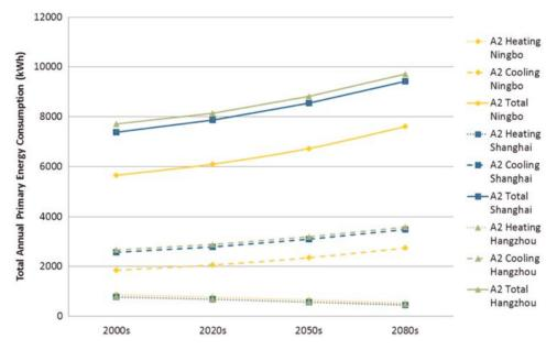
Figure 13. Comparison of heating and cooling demands for the 'control' office room in Ningbo, Shanghai and Hangzhou.
