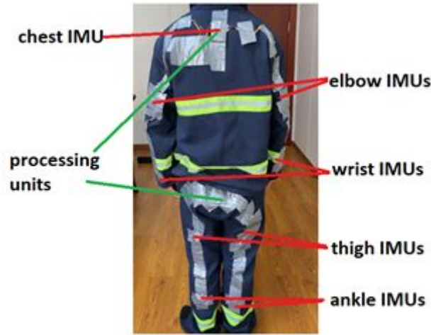
Figure 3.7: Placement of motion sensors that are mapped to the body parts where the motion data are critical for fall-detection computation.
