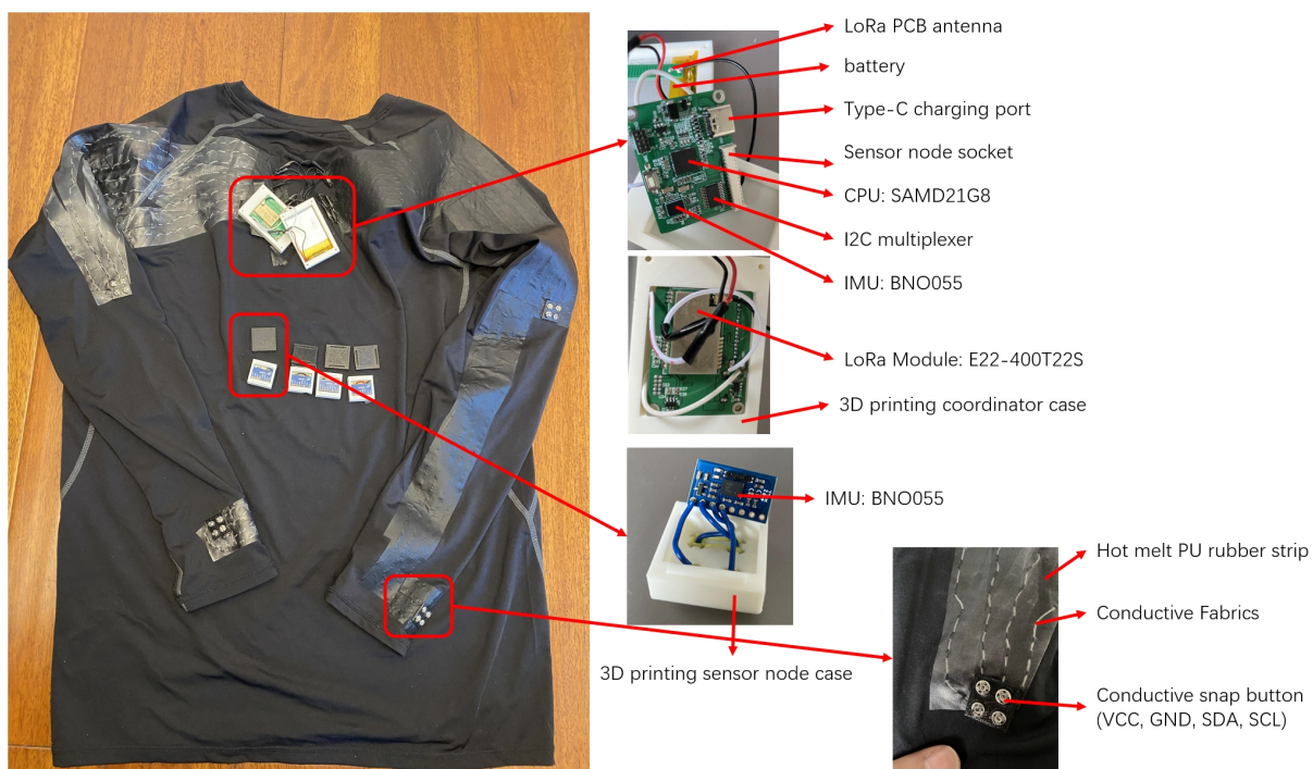
Figure A.2: Interim version of the wearable prototype with conductive fabrics developed in 2022.
