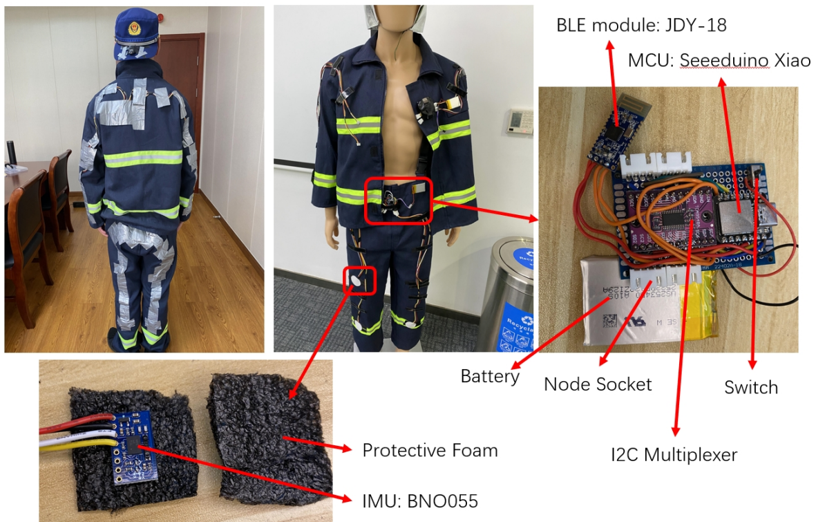
Figure A.1: First version of the wearable prototype with wired connections developed in 2021.
