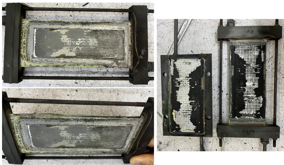
Figure 5.11. Macro morphology of Cell5.3 after durability test
