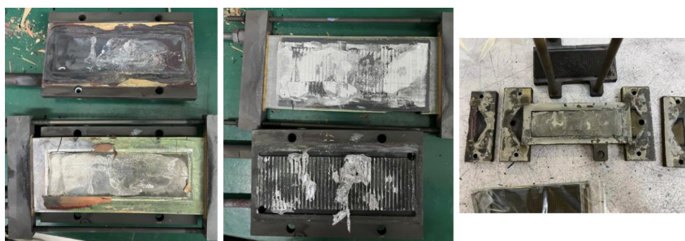
Figure 5.12. Macro morphology of Cell5.4 after durability test
