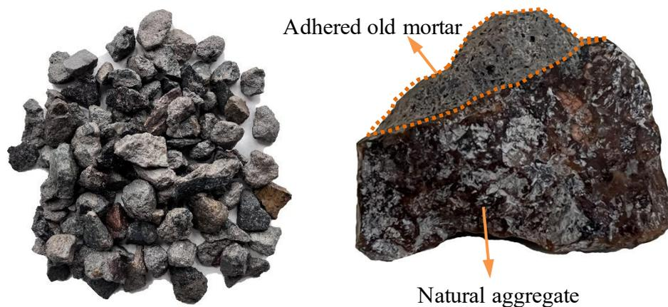
Fig. 1.2 Recycled concrete aggregate
