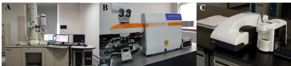
Figure 2.1: The photos of the equipment A) Transmission electron microscopy (TEM, JEOL. 2100, Tokyo, Japan); B) Confocal microprobe Raman system (Renishaw inVia Reflex, Wolton-under-Edge, U.K.); C) Zeta particle size analyzer (Malvern, England).
