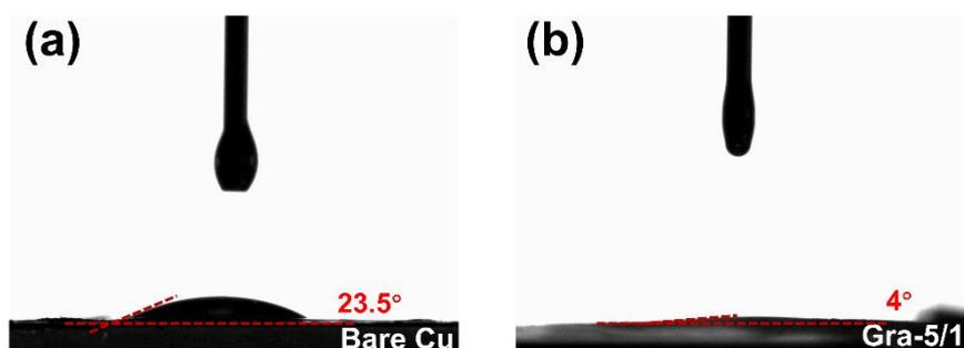
**Figure 6.11.** Contact angles of electrolyte toward (a) Cu foil and (b) Gra-5/1.
