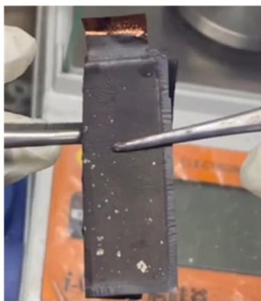
**Figure 6.15.** The optical photograph shows the flexibility of Gra-5/1 after 100 cycles of deposition/dissolution in a full pouch cell.
