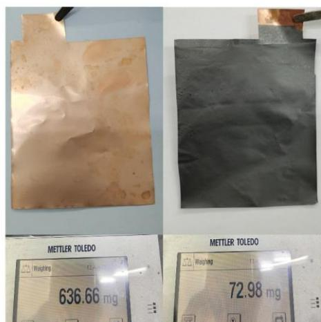
**Figure 6.4.** Optical photographs showing the appearance and weight of bare Cu (left) and Gra-5/1 (right).
