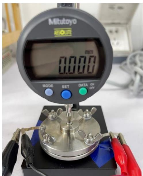
**Figure 2.3.** *In-situ* swelling test cell.
