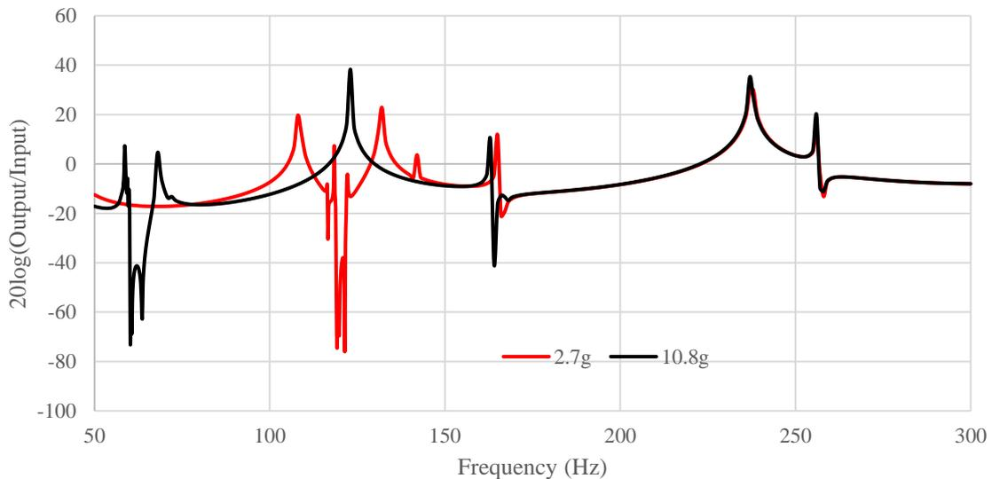
Figure 7. Frequency response of plate when the mass magnitude is 2.7g (Red line) and 10.8g (black line).
