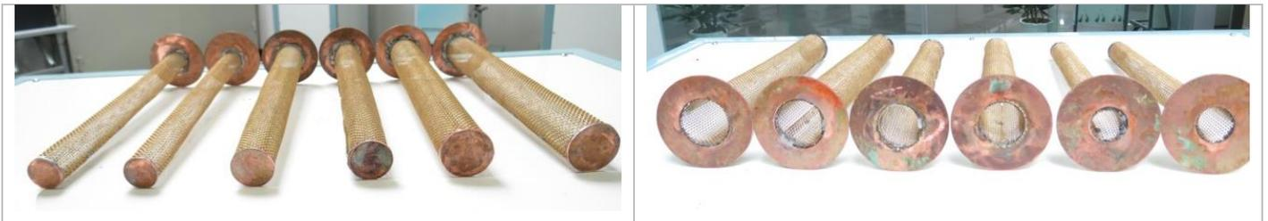
Figure 5 Different Dimensions of the Copper Cylindrical Mesh Pipes Fabricated for the Experiment
