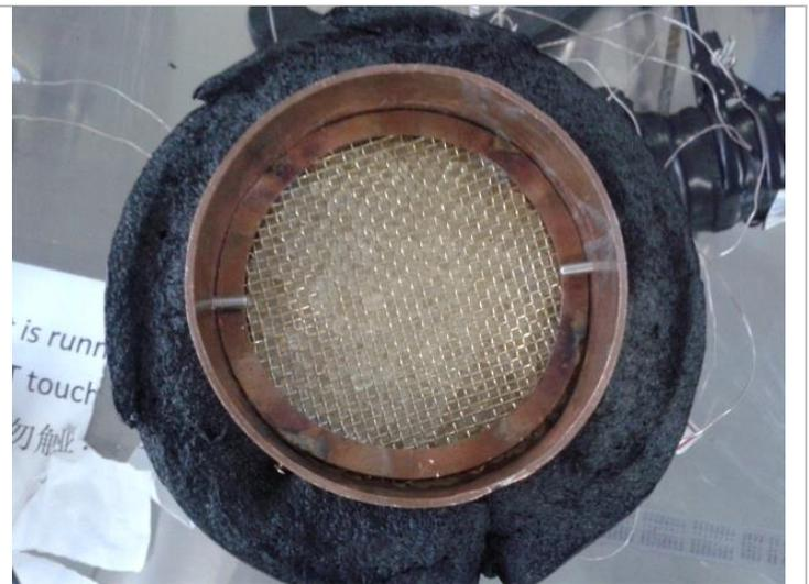
Figure 7a Packed Bed with Annulus Insert and Thermocouple (TC) Probes
