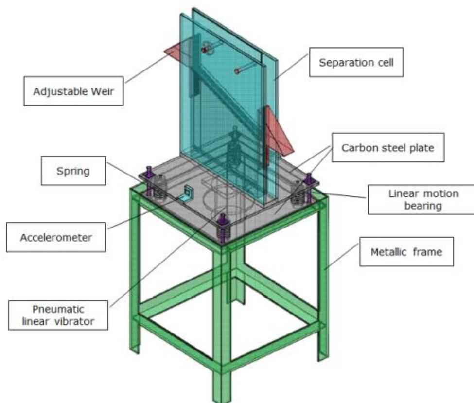
Figure 1. The design of a novel vibratory separator
