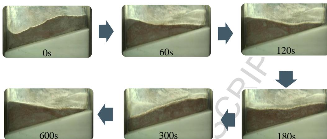
Figure 8. Vibratory separation of copper and polypropylene particles (0% w/w talc ,
