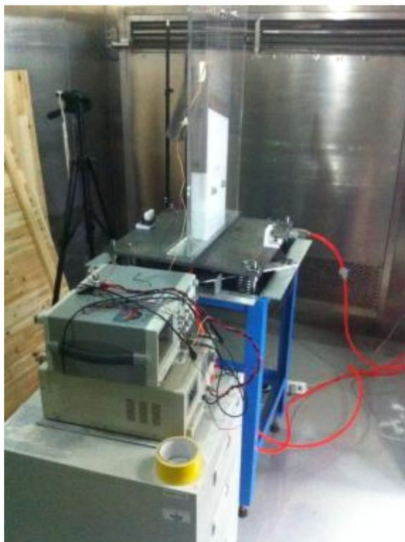
Figure 6 Vibratory separator in Edeson EWR-30S-A Environmental chamber
