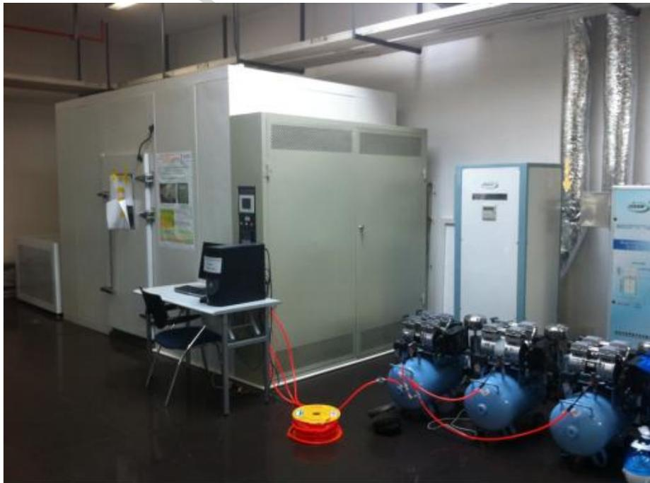
Figure 5 Experimental set-up with Edeson EWR-30S-A Environmental chamber
