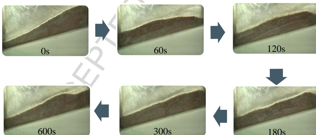
Figure 9. Vibratory separation of copper and polypropylene particles (0.1% w/w talc as
