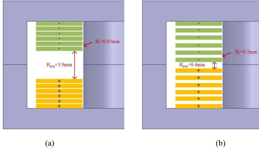
Fig.5.2.11 Two winding arrangements for the validation of the proposed, (a) Insulation thickness  $h_i = 0.05$  mm, thickness of the gap between two coils is  $h_g = 3.9$  mm. (b) Insulation thickness  $h_i = 0.2$  mm, thickness of the gap between two coils is  $h_g = 0.4$  mm.
