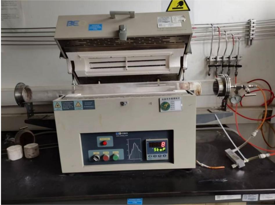
**Figure 3. 1.** BEQ horizontal high-temperature tubular furnace.
