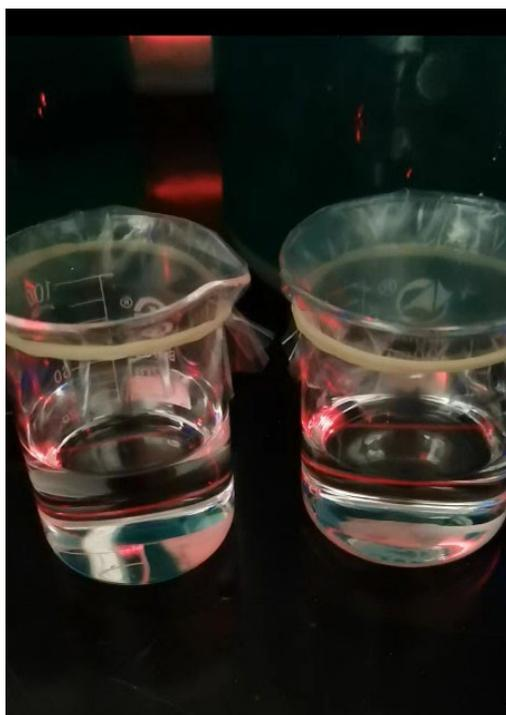
**Figure 5. 6.** Transparent  $B_2O_3$  ethanol sol with the light scattering by laser beam.
