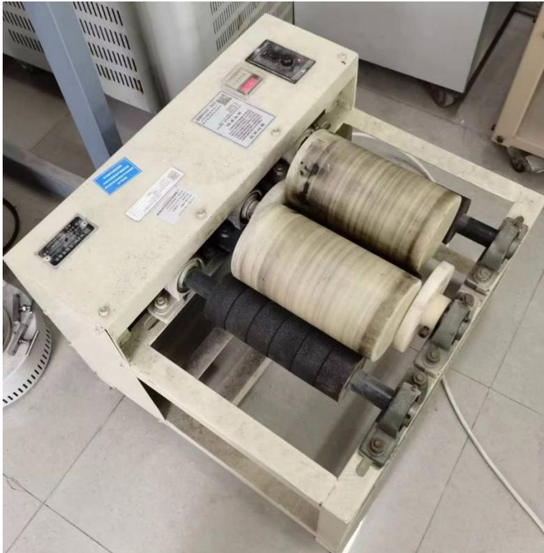
**Figure 3. 2.** WZM 1.5 L double-tank ball mill machine.
