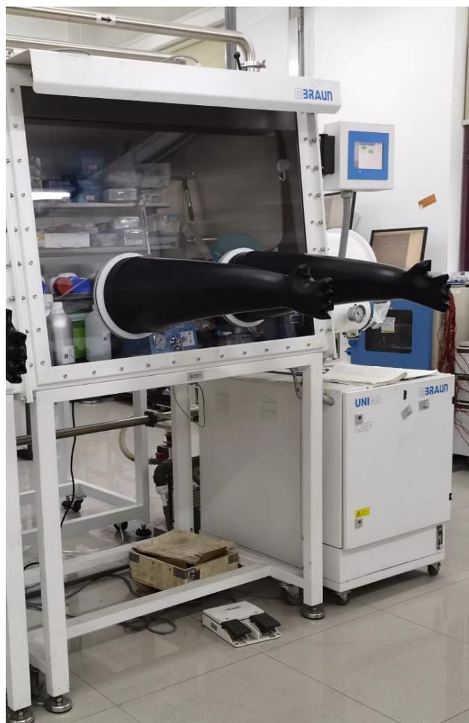
**Figure 3. 3.** MBRAUN UNI-lab glove box workstation.
