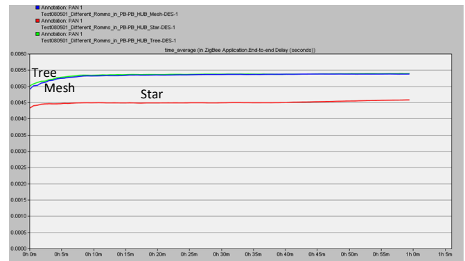
Fig. 6. End-to-end delay of different topologies in the service center.
