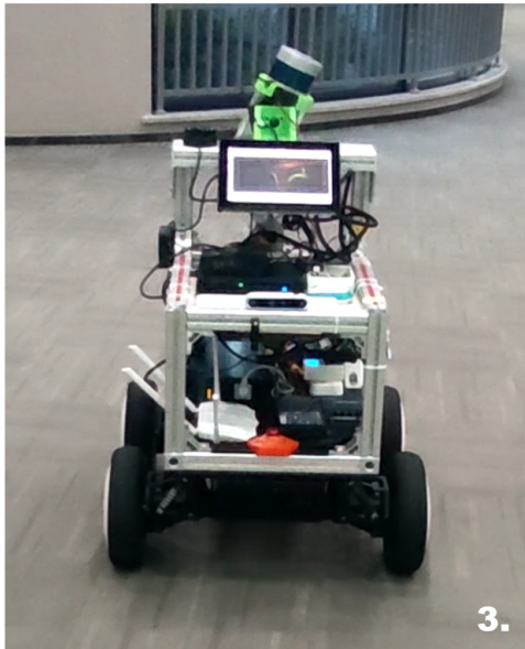
Figure 5.8: RoboBIM automatic scanning robot undergoes fully functional testing at IAMET 2f at UNNC. Fig.5.8.1-4 demonstrate the robot's continuous autonomous motion.
