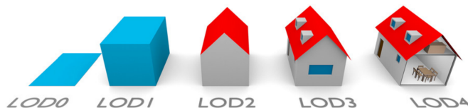
Figure 1.2: To better describe the geometric features of BIM, Level of Detail (LoD) was proposed by CityGML [2] to describe the geometric feature richness of BIM. the geometric feature model described by LoD is usually considered to be 2D and 3D BIM [3].
