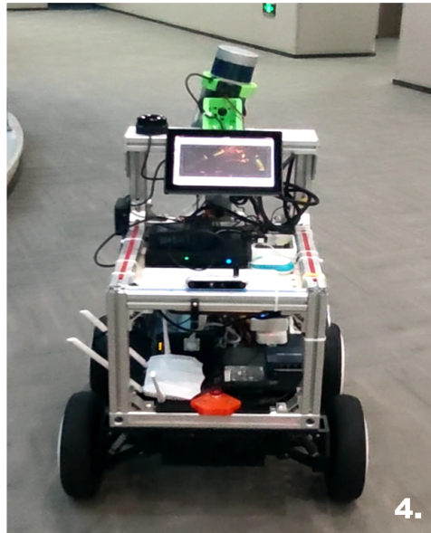
Figure 5.8: RoboBIM automatic scanning robot undergoes fully functional testing at IAMET 2f at UNNC. Fig.5.8.1-4 demonstrate the robot's continuous autonomous motion.
