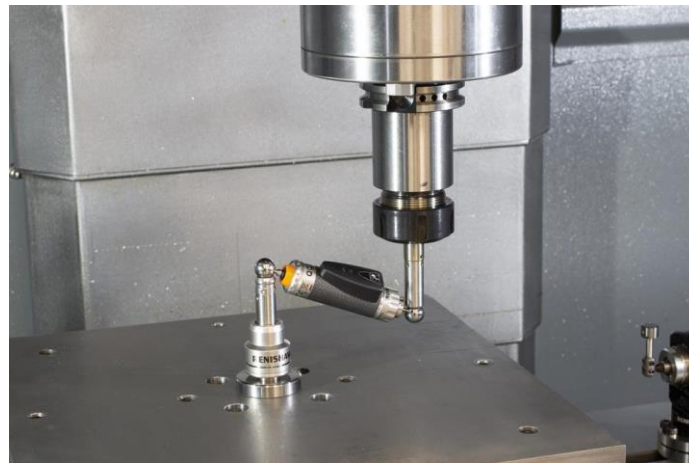
Figure 8 Calibration from Renishaw QC20 ball-bar
