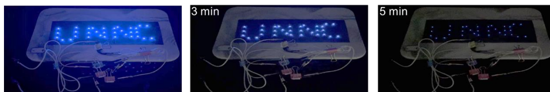
Fig. 6.11 Digital photos of the character of “UNNC” composed of 33 blue LED light driven by four ASSC devices connected in series.
