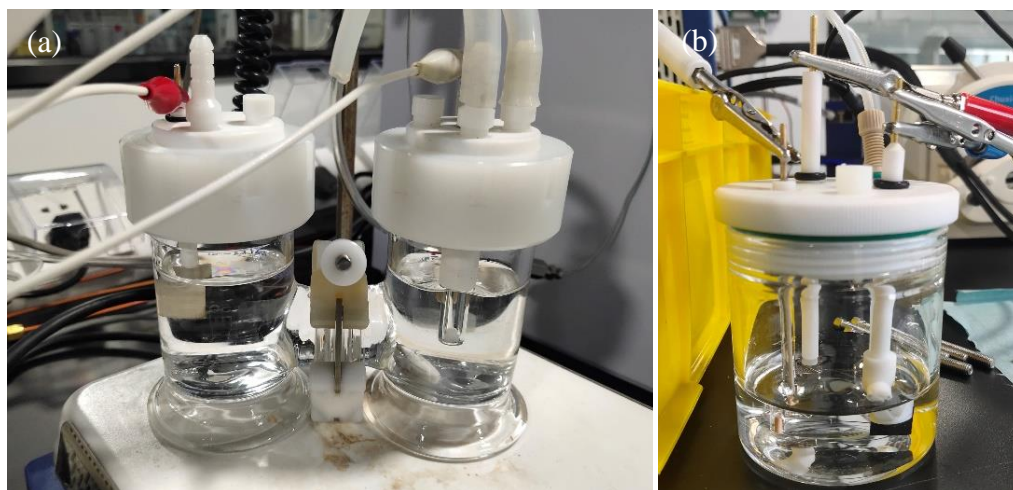
Figure 3.1 (a) H-type electrolytic cell and (b) common sealed electrolytic cell.
