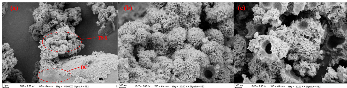
Figure 1. The images of BC@TNS before adsorption (a), enlarged view with details (b), and after adsorption (c).
