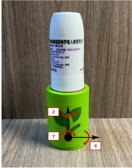
Figure 7. 3: Axial directions of gyrometer.
