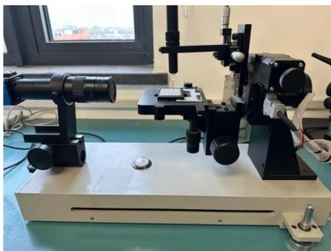
Figure 3.1 Contact angle test machine
