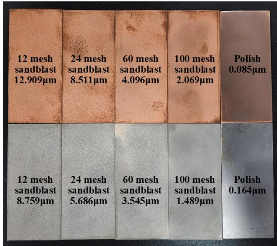
Figure 42: Sample copper and stainless steel plates with different surface roughness
