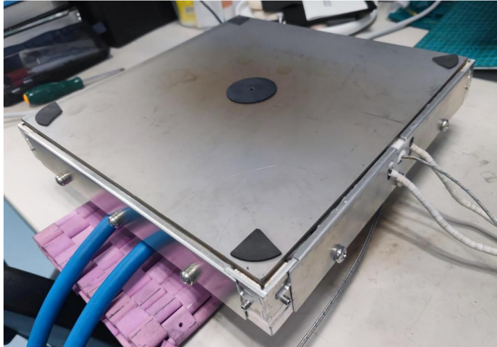
Figure 36: Manufactured and assembled substrate system with 4mm stainless steel plate and waiting for temperature testing
