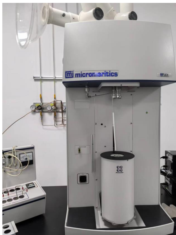
Figure 3.6 Image of the BET instrument.
