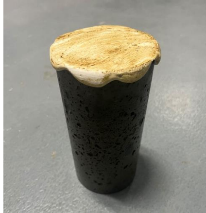
Figure 12. Concrete cylinder for compressive strength test
