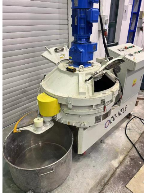
Figure 9. Concrete mix machine
