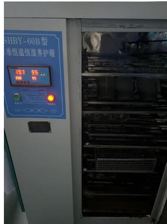
Figure 11. Concrete curing container
