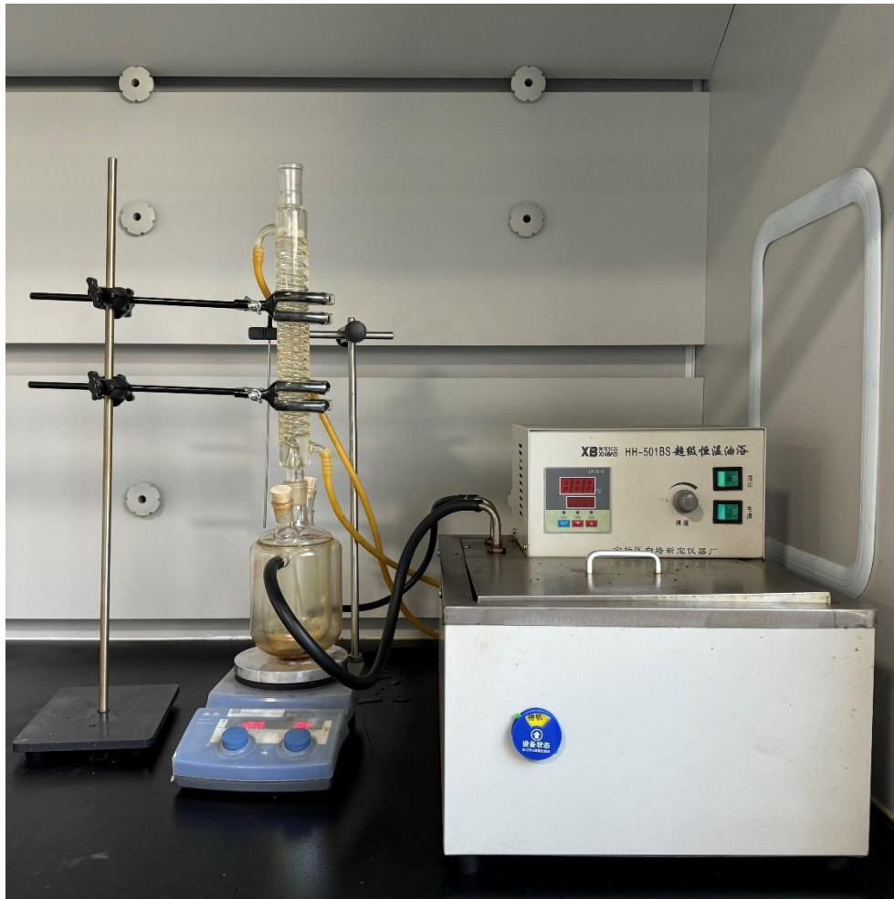
Figure 3.1 Oil bath device (synthesis temperature = 80°C, synthesis time = 24 h).
