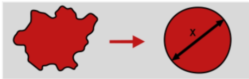
Figure 3. 13 Schematic of diameters derived from the equivalent circle(Li et al., 2005).
