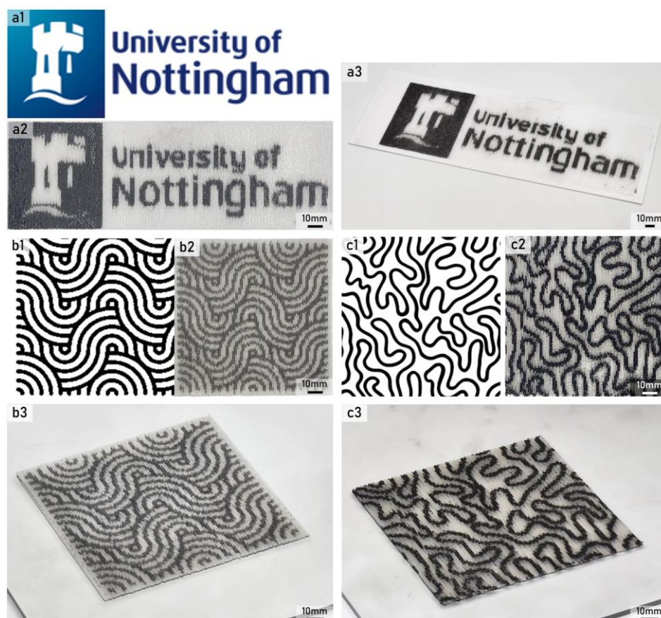
Figure 4-3 Exemplars of 2D pattern prints with the slicing software that considered advance distance and in-line adjusting nozzle speed. a) Logo of University of Nottingham; b) 2D print of repeat pattern; c) 2D print of random patterns.
