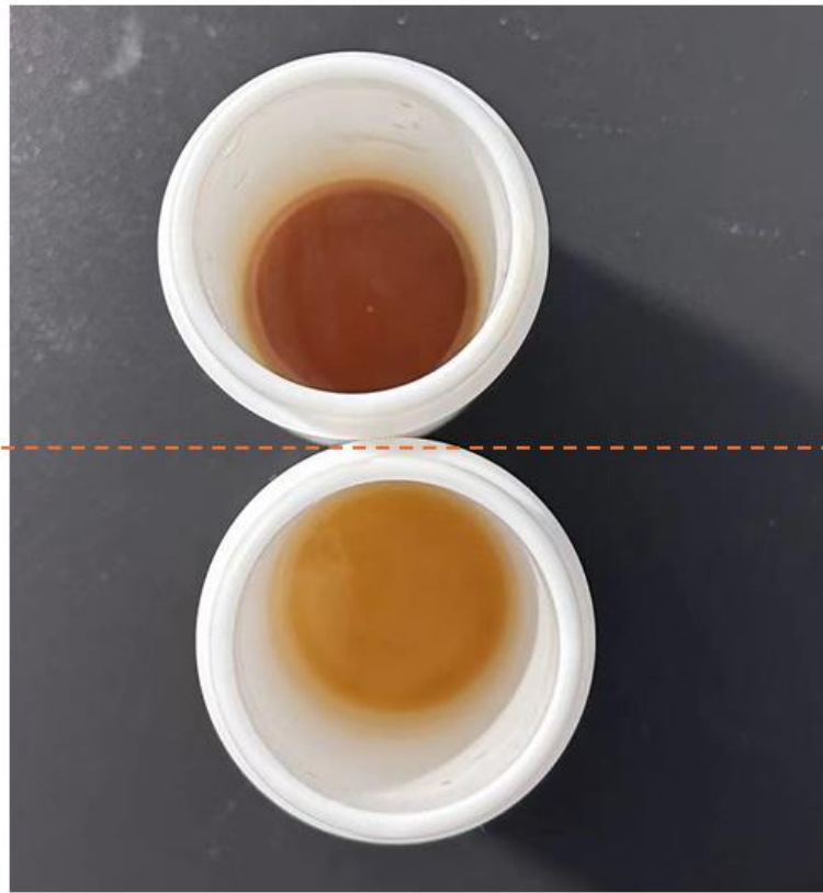
Figure S4 The gels at the bottom of reactor after crystallisation (Two samples were synthesised in the presence of 0.02M SPS, and the sample above the dashed line utilized 1.3wt% CNCs, whereas the sample below the dashed line utilized 1wt% CNCs).
