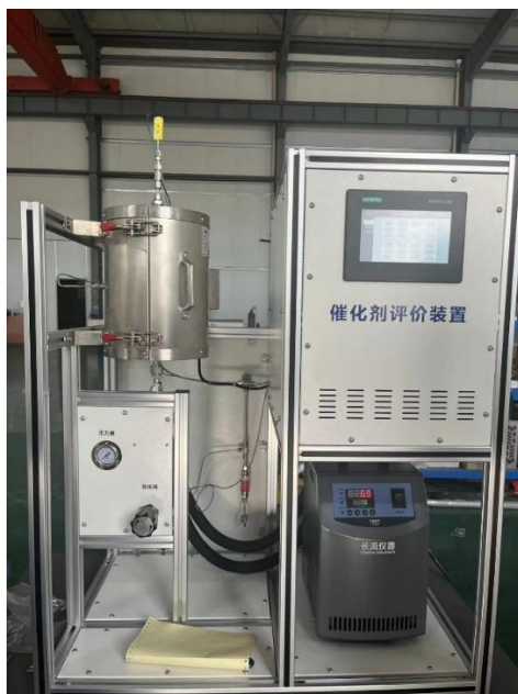
Figure 3.7 The fixed-bed reactor for catalytic tests.
