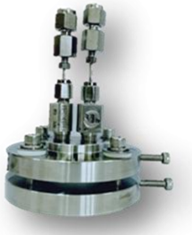
Figure 3-3 Photographic view of the experimental setup of battery mold.
