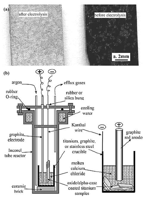
Fig. 2. (a) Optical scanning image of an alpha-case covered Ti-6AI-4V foil (right) before and (left) after electro-reduction in molten CaCl<sub>2</sub> at 3.0 V and 950°C for 1 h. (b) Reactor and electrolytic cell for removal of the alpha-case on titanium and alloys in molten CaCl<sub>2</sub>, showing (left) a sample suspended in molten salt and (right) more samples placed at the bottom of the crucible. Reprinted from<sup>69</sup> with permission.
