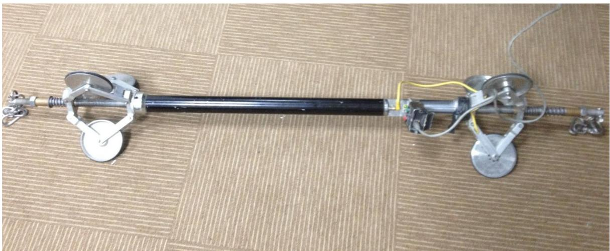
Figure 15 The Ductrunner pipeline mapping system.
