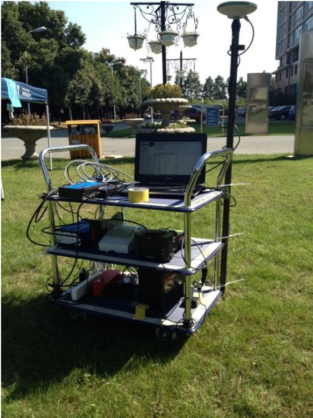
Figure 2 Rovers fixed on a trolley.
