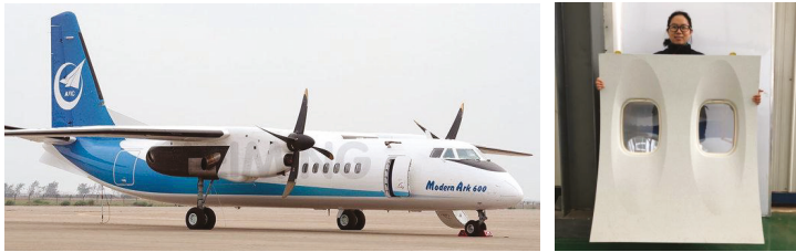
Figure 5. MA600 airplane and the composite side panel made of AGMP3600/honeycomb sandwich composites (Photos courtesy of Fangbo Ding, AVIC XAC, Commercial Aircraft Co., Ltd.).
