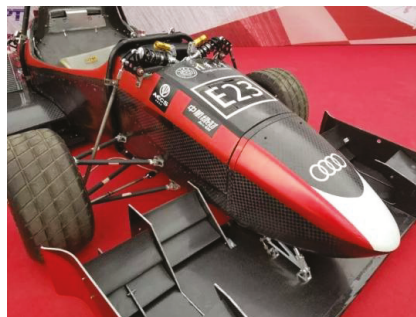
Figure 6. Electric race car, its body was manufactured using AGMP3600/honeycomb sandwich composites.
