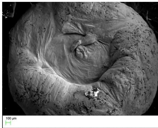
Figure 53. SEM image of a solidified droplet before the end of the oscillation.
