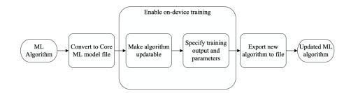
Figure 5.11: ML algorithm deployment and update
