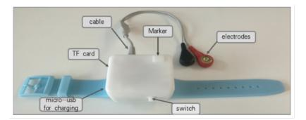
Figure 4.5: GSR sensor developed by Xinhua Net, sourced from S. Li (2019)
