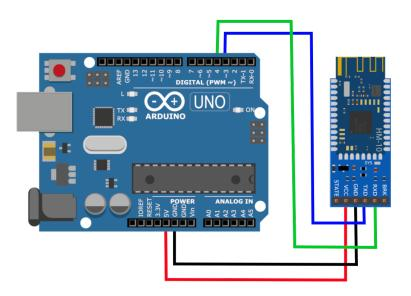
Figure 4.13: AT-09 BLE module wiring diagram, sourced from Hrisko (2019)
